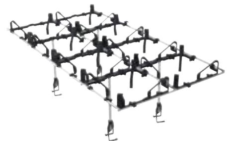
The new support frame provides additional hold. As and when required, it is placed on top of the injector module, providing a secure hold to even large items of laboratory glassware in a vertical and protected position.
