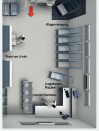
A typical room layout for a barrier wash system with clean and dirty sides
