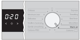
■ Touch the < or > sensor control until the required duration lights up.
