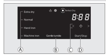
The A-D sensor controls react to fingertip contact. If a sensor control is illuminated, it can be selected.
