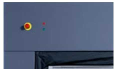
Programme sequence monitoring via LEDs on the clean side (on machines with Octo blue external finish)
