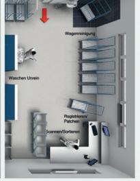
A typical room layout for a barrier wash system with clean and dirty sides
